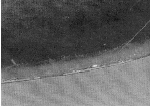
Fig. 7. Silicate deposit after evaporating solution containing 14, PPM Si from "glass fines" and water mixture exposed 24 hours at 72°F; after 5% acetic acid wash; 200X
