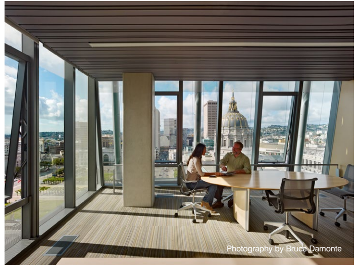
The 13-story building, which is LEED certified at the Platinum level, has an open office design and raised floors that enhance ventilation, while IGUs incorporating Solarban ® 70XL glass over Starphire ® glass allow natural light to indirectly penetrate work spaces.
