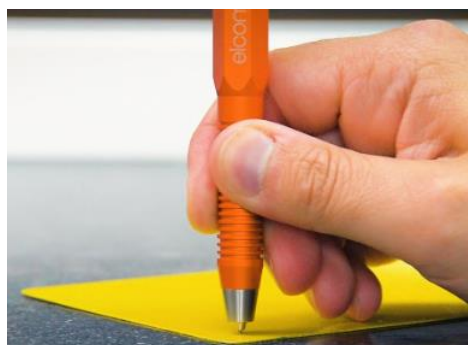
Drag Sclerometer Across Painted Surface Damage to Paint Should Not be Visible from Unpainted Side
