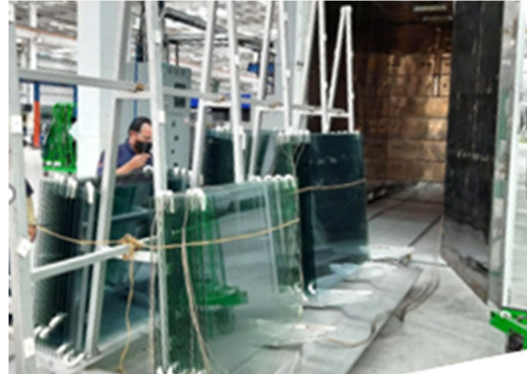
An example of a heat soak oven glass load that has thermocouples placed to monitor the glass temperatures.
