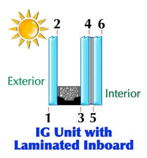
Table 4 shows a few examples of Vitro products used in an IGU with inboard laminated glass construction that will meet or exceed the VLT requirements of the marine protection ordinance. The laminate in this case is constructed with a standard PVB interlayer.
