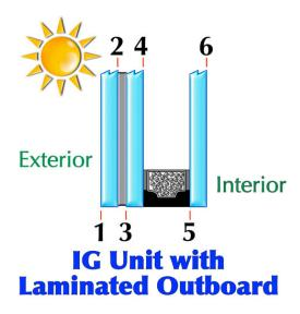
Table 5 shows a few examples of Vitro products used in an IGU with outboard laminated glass construction that will meet or exceed the VLT requirements of the marine protection ordinance. The laminate in this case is constructed with a standard PVB interlayer.
